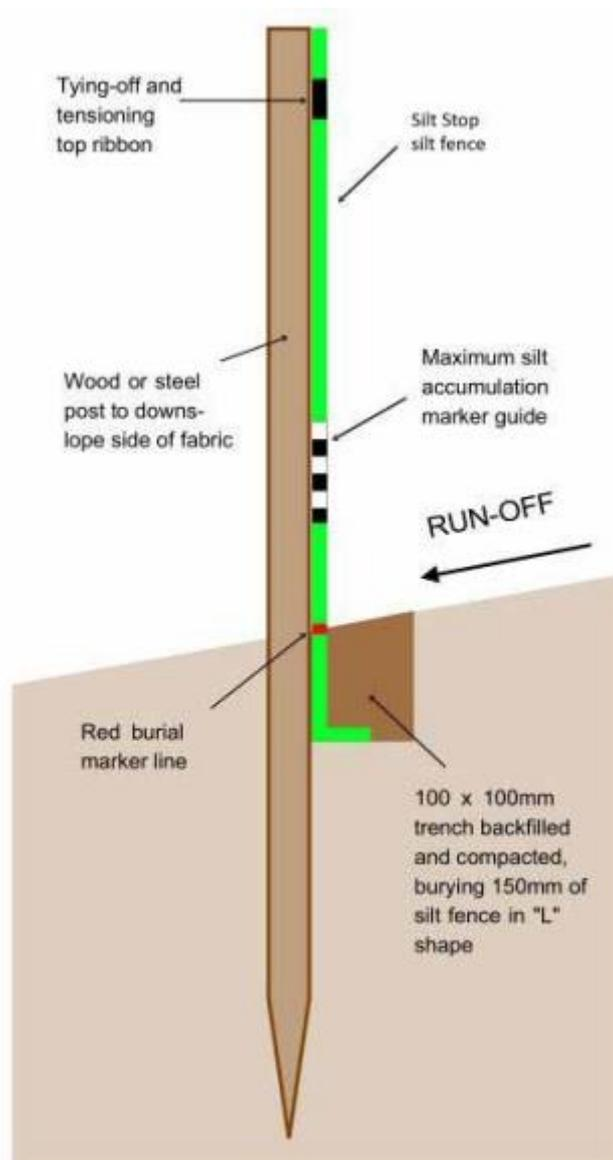
Figure 7-12 Silt Fence Cross Section [Source Hy-Tex Terrastop Silt Fence Construction Methods]
