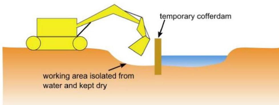
Figure 7-15: Partial Isolation Cofferdam
