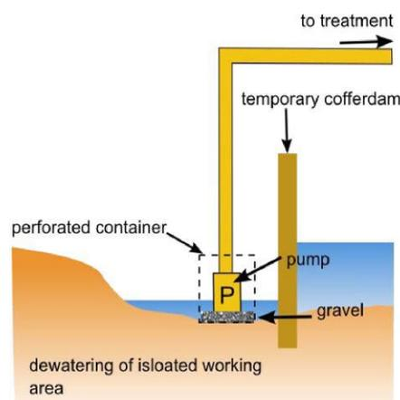
Figure 7-9 Submersible Pump on a gravel base and perforated container [Source SEPA Engineering in the Water Environment Good Practice Guide Temporary Construction Methods]
