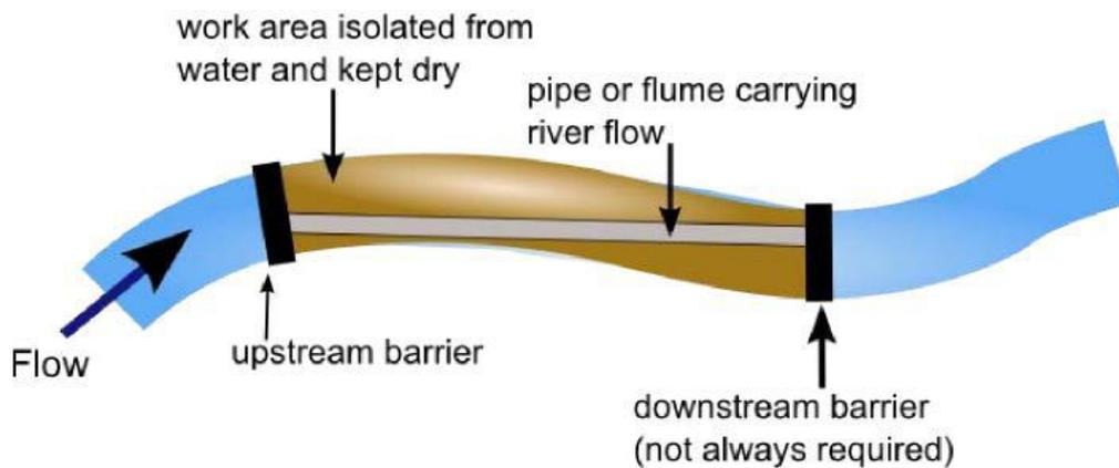
Figure 7-14: Full Isolation Gravity/Flume pipe
